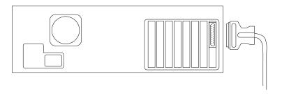
3. Attach the other end of the cable to either of the identical SCSI ports on the back of the Scanner. Seat the connector firmly and pinch the thin wire clamps shut.
